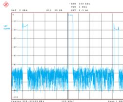
Fig. 6-69 Transition to display in time domain. Pulse duration of 500 μs and period of 2 ms can be clearly recognized
